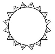
When handling 'sticky' dust, a very high-pressure differential can be experienced across the filter media. This situation can deform the pleats under operation and will result in a sharply decreased filter area. For such situations, it is recommended that special Clyde-Filtercorp pleat-separators are used.
