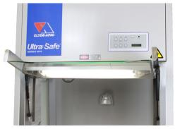
To open the window, pull it firmly outwards. It will support itself in the open position. To close the window, push it down towards the closed position. If the viewing window is opened when the cabinet is running, a boost mode, which activates maximum exhaust airflow and the alarm system, is automatically selected.
